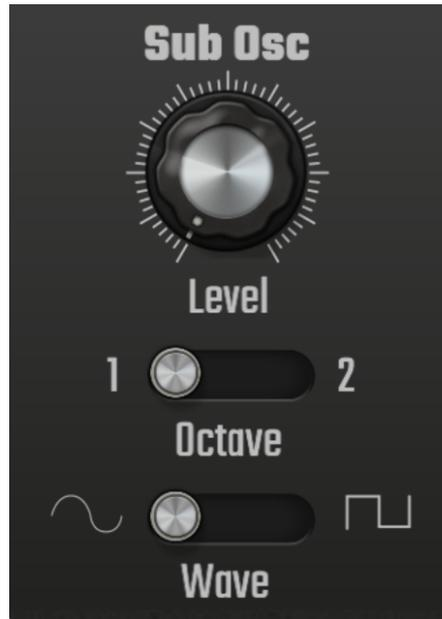
As already mentioned, there is a sine wave in the FM panel but Evolution One also offers a sine or square wave sub-oscillator. The sub-oscillator gives you an additional oscillator which plays at a fixed one or two octaves below the note triggered. This can give you a fuller, bass-rich sound when required.
