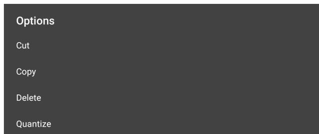
As you can see, these options allow you to **Cut** (remove and copy to clipboard), **Copy** (copy to clipboard), **Delete** and **Quantize** (snap to exact musical increments of the tempo). When Quantize is selected a further dialog will open allowing you to tailor the quantization to your requirements as described [here](#).
