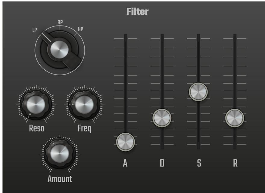
The **Filter** section of the Envelope page allows you to filter out frequencies from your synth sound and also has its own Filter Envelope to control how the Filter effects the sound's frequencies over time.
