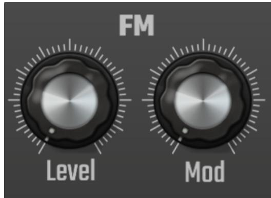
FM stands for Frequency Modulation. Evolution One provides what is referred to as an FM pair. This comprises of a Carrier signal (the signal to which the modulation is applied) and a Modulator (whose frequency modulation index modulates the frequency of the carrier signal). In this case, the process generates side band harmonics as the Mod is increased, resulting in a richer, brighter output waveform.
