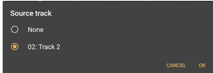
The **Source track** is the track which will be monitored by the compressor and will be used to trigger the compression being applied when its signal goes above the Threshold set. Pressing **OK** will then open the Source block dialog, below.
