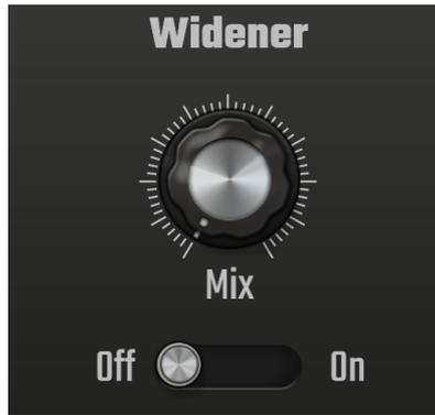
As explained in the [Auto Pan](#) section below, the Evolution One synth sound exists in a stereo sound field. The **Widener** is a clever effect which spreads and widens the stereo effect of the selected preset.
