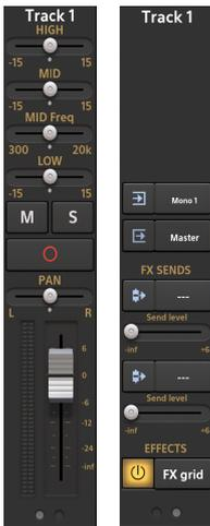
. The Channel Strip gives you a range of controls over the currently selected track and allows you to access the FX (effects) Grid for audio and instrument tracks. These controls are shown across more than one Channel Strip page. For more details about the Channel Strip for audio tracks, see [here](#). For more details about the Channel Strip for instrument tracks, see [here](#).
