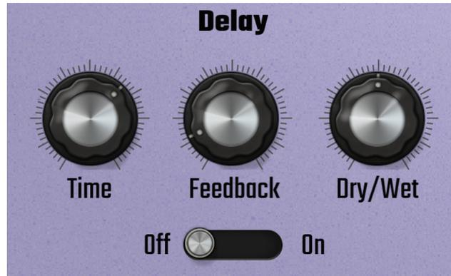
Delay effects record the incoming sound and replay it after a time delay. Depending on the feedback time specified, the sound continues to be delayed and replayed, each time getting quieter until silence is reached. They can be used to create echo effects but they don't really simulate natural phenomena in the way that reverbs do (though reverbs *are* delay based effects). They are very creative tools and widely used, in their various forms, within music production and sound design.
