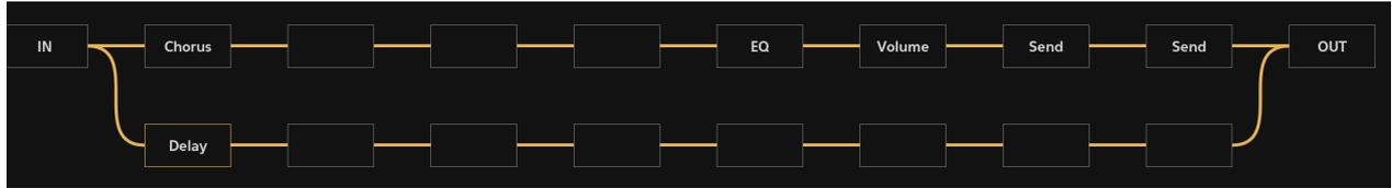
So here, using parallel processing, the original 'clean' signal/audio is being sent through the Chorus effect at the same time as a *copy* of that clean signal is also being sent through the Delay effect. As it is shown here, the two copies remain separate until they are both heard together at the Output. If though, for example, you wanted to apply *the same* Reverb effect to both the 'chorused' and the 'delayed' signals, you could then simply route the delayed signal back up like this.
