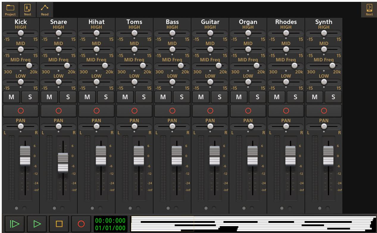
This screen displays the Channel Strips of all of the tracks in your project next to each other in the manner of a mixing console. If there are more tracks in the project than will fit on the screen all at once, you can swipe to the left over the names on the channel strips to access the channel strips of tracks which are not displayed initially.
